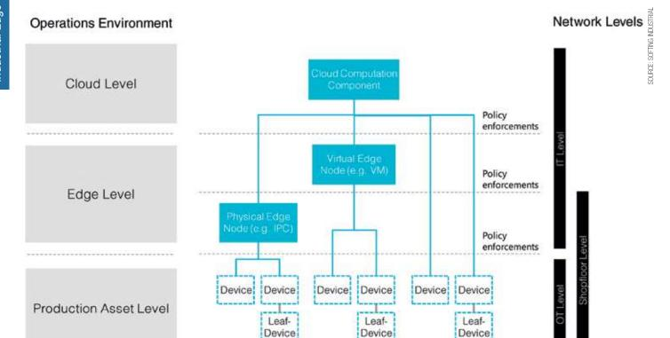
The three levels of the Industrial IoT solution: production assets, edge and central platform.
