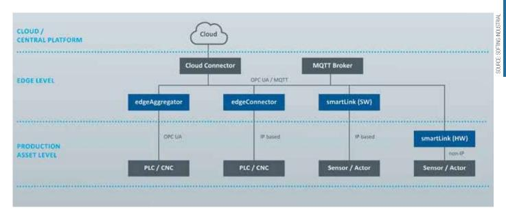
Softing products for integrating machine connectivity into the edge level of an Industrial IoT solution.
